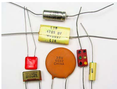
Figure 8.4 These are some typical capacitors used in electronic devices. A capacitor's size is not necessarily related to its capacitance value.
