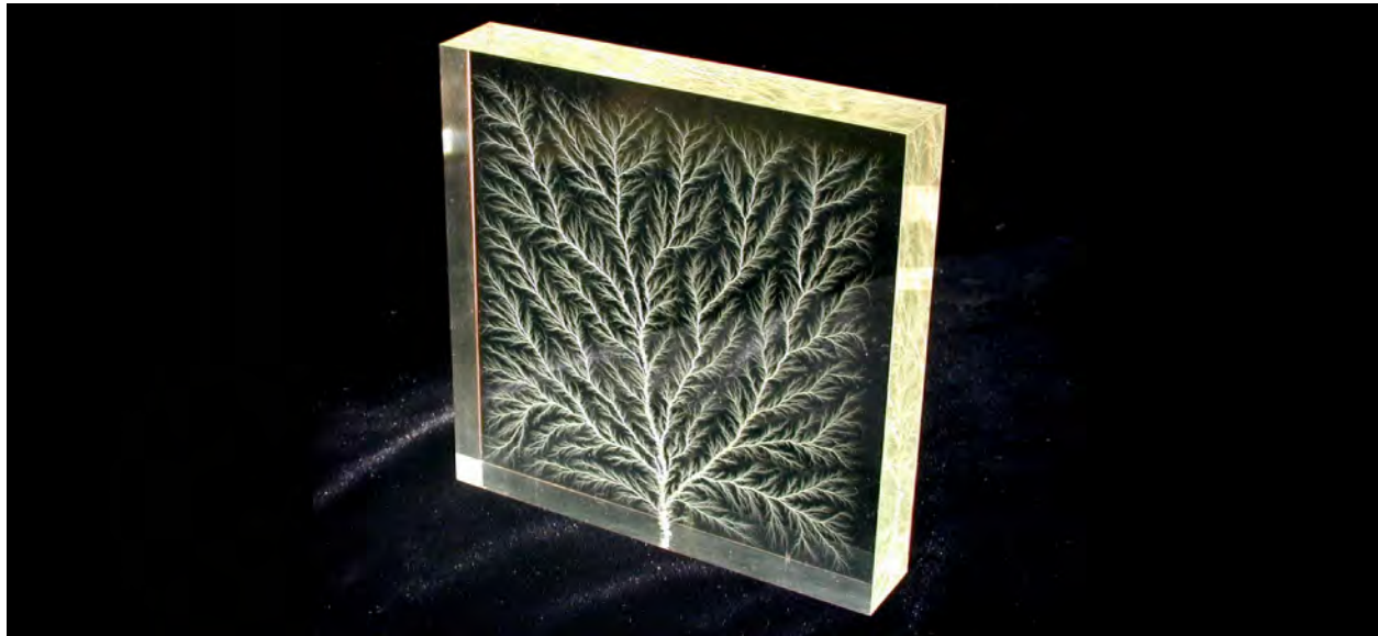
Figure 8.1 The tree-like branch patterns in this clear Plexiglas® block are known as a Lichtenberg figure, named for the German physicist Georg Christof Lichtenberg (1742–1799), who was the first to study these patterns. The “branches” are created by the dielectric breakdown produced by a strong electric field. (credit: modification of work by Bert Hickman)
