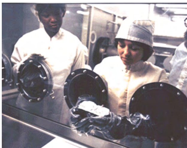
Figure 9.4 Handling Moon Rocks. Lunar samples collected in the Apollo Project are analyzed and stored in NASA facilities at the Johnson Space Center in Houston, Texas. Here, a technician examines a rock sample using gloves in a sealed environment to avoid contaminating the sample. (credit: NASA JSC)
