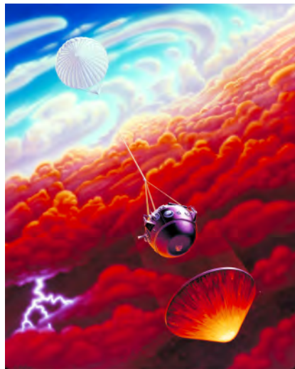
Figure 11.3 Galileo Probe Falling into Jupiter. This artist's depiction shows the Galileo probe descending into the clouds via parachute just after the protective heat shield separated. The probe made its measurements of Jupiter's atmosphere on December 7, 1995. (credit: modification of work by NASA/Ames Research Center)
