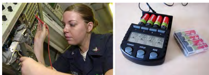
Figure 21.13 These two battery testers measure terminal voltage under a load to determine the condition of a battery. The large device is being used by a U.S. Navy electronics technician to test large batteries aboard the aircraft carrier USS Nimitz and has a small resistance that can dissipate large amounts of power. (credit: U.S. Navy photo by Photographer's Mate Airman Jason A. Johnston) The small device is used on small batteries and has a digital display to indicate the acceptability of their terminal voltage. (credit: Keith Williamson)
