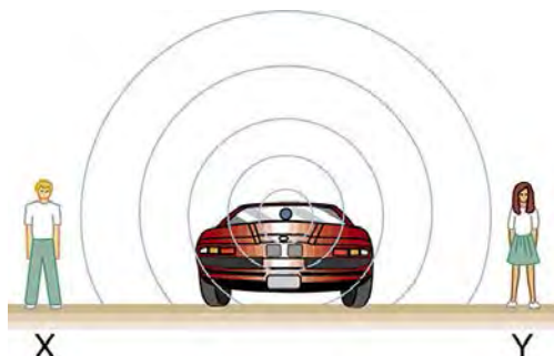
Figure 17.14 Sounds emitted by a source spread out in spherical waves. Because the source, observers, and air are stationary, the wavelength and frequency are the same in all directions and to all observers.
