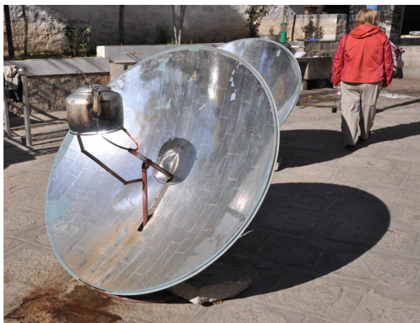
Figure 3.17: A parabolic reflector used to boil water in the kettle that is at the focal point of the dish, in Lhasa, Tibet.
