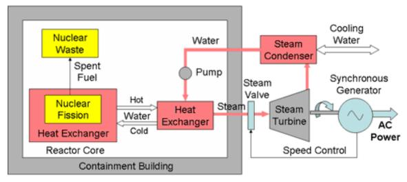
Pressurised Water Reactor (Two Stage Heat Transfer)
