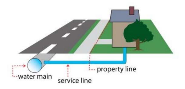
It is also important to point out in this particular picture there is no water meter or valves connecting the pipes. However, it is a nice reference for illustration purposes.
