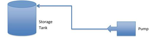
between the pump and tank too. When the level in the storage tank gets low, the pump would need to be turned on to refill the tank. While the tank is filling, customers might be connected to the pipe leading to the tank and use some of the water while it makes its way to the tank. Once the tank is full the pump would then be turned off.
