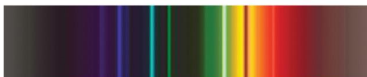
High-pressure Na spectrum (350-700 nm)
