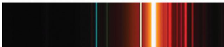
Low-pressure Na spectrum (350-700 nm)
