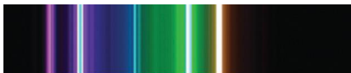
Hg vapor spectrum (350-700 nm)
