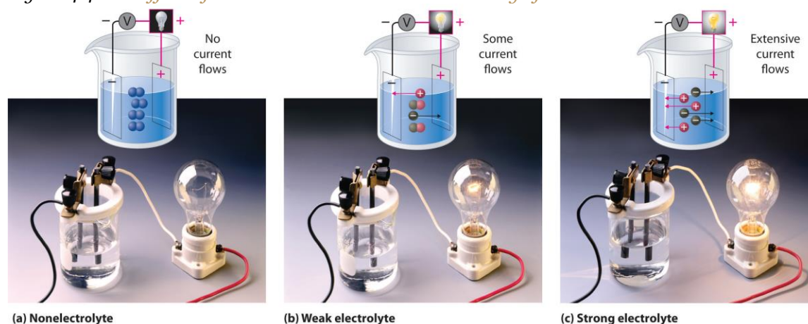
Figure 4.4 The Effect of Ions on the Electrical Conductivity of Water
