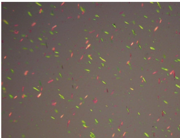
Fig. 7.4 Birefringence of the CR bound on SWNT (polarized light microscopy)
