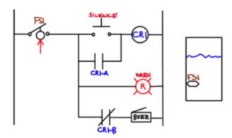
Describe the behavior of the above circuit if a NO pressure switch and a NO temperature switch are placed in parallel with the NC-HO FS1.
