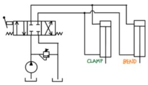
Describe the operation of this multi actuator hydraulic circuit making use of a sequence valve on the cap end of the bend cylinder. Assume the set value of the sequence valve is 400psi and the main pressure relief valve is set to 800psi.
