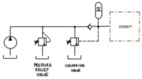
Use this hydraulic circuit and diagram of two pilot darts to describe the general operation of a differential unloading relief valve.
