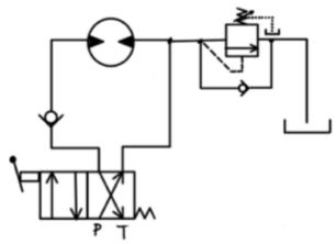
Describe how these two sequence valves can be used to brake a bidirectional hydraulic motor.
