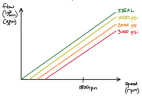
Given a pump with a fixed displacement of .35CIR at ideal conditions, calculate flow rate in gpm if the pump was driven at exactly 1800 rpm.
