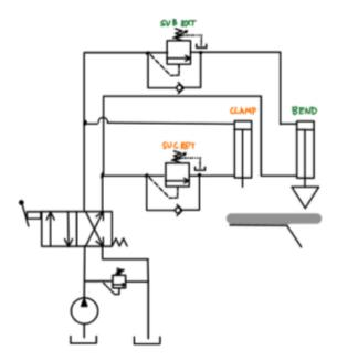
Describe the operation of this hydraulic circuit making use of a sequence valve with an external remote pilot used to coordinate two separate actuators (stabilizer boom and crane) using two independent directional control valves.
