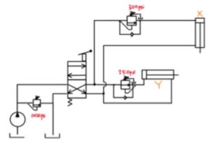
Discuss how set values of the pressure reducing valve, sequence valve, and main pressure relief valve influence the proper functionality of the above system.
