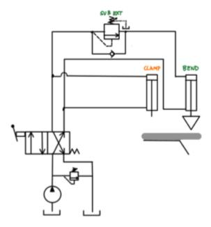
Describe the operation of this multi actuator hydraulic circuit making use of a sequence valve on the cap end of the bend cylinder and another sequence valve on the rod end of clamp cylinder.
