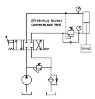
Describe the operation of this circuit making use of an internally and externally piloted counterbalance valve used to lower a heaving mold, forming piece or platen. Comment on the behavior of this system during lowering and the maximum downwards force it is capable of generating.
