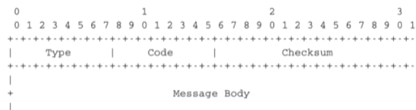
Fig. 3.55: ICMP version 6 packet format
