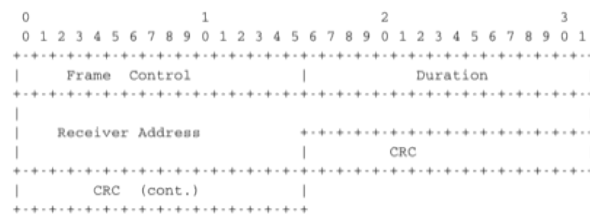
Fig. 3.98: IEEE 802.11 ACK and CTS frames
