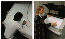
Vector digitizing with a tablet (left); raster digitizing with a drum scanner (right) (USGS).
