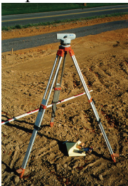
A level used for determining elevations.
