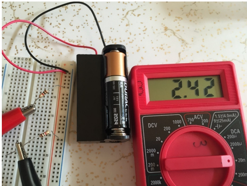
Figure 1.8: Circuit showing current measured with a Multimeter.
