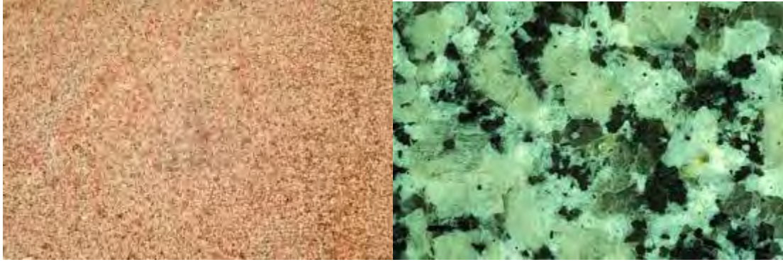
Figure 23: The fine grained rock on the left contains lots of small grains of quartz. The coarse grained granite on the right also contains quartz, but in larger grains.
