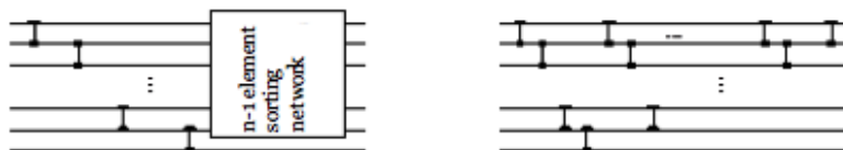
Exhibit 17.18: Selection sort leads by induction to the sorting network on the right.
