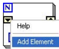
Figure 5.24 Adding Shift Register Elements
