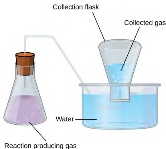
Figure 9.21 When a reaction produces a gas that is collected above water, the trapped gas is a mixture of the gas produced by the reaction and water vapor. If the collection flask is appropriately positioned to equalize the water levels both within and outside the flask, the pressure of the trapped gas mixture will equal the atmospheric pressure outside the flask (see the earlier discussion of manometers).
