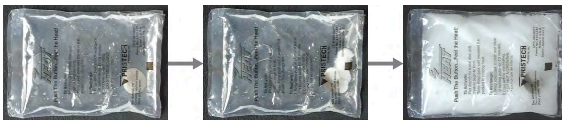
Figure 11.18 This hand warmer produces heat when the sodium acetate in a supersaturated solution precipitates. Precipitation of the solute is initiated by a mechanical shockwave generated when the flexible metal disk within the solution is “clicked.” (credit: modification of work by “Veleta”/Wikimedia Commons)
