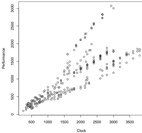
Figure 3.1: A scatter plot of the performance of the processors that were tested using the Int2000 benchmark versus the clock frequency.
