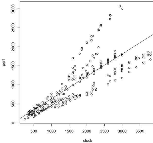
Figure 3.2: The one-factor linear regression model superimposed on the data from Figure 3.1.
