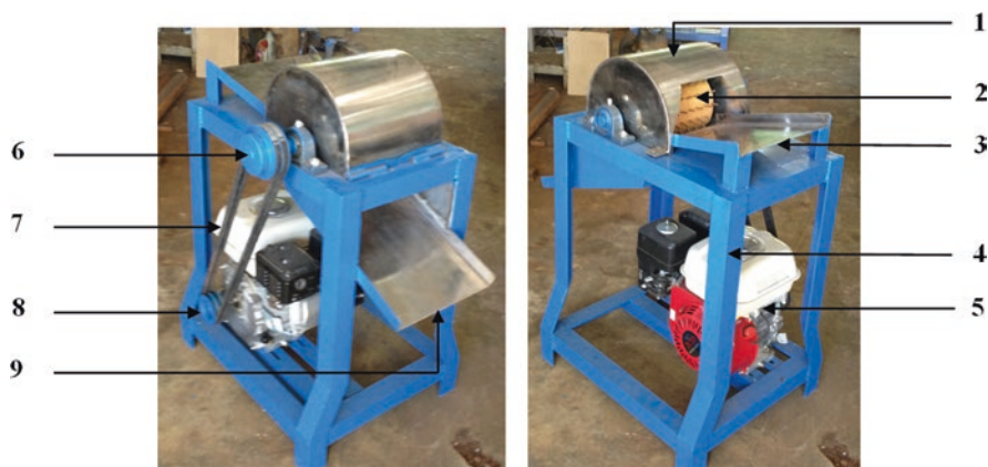
Fig. 17.2 Overall structure of cylinder-type sago rasping machine. (1) Cylinder cover, (2) rasping cylinder, (3) input hopper, (4) main frame, (5) gasoline engine, (6) cylinder pulley/driven, (7) V-belt, (8) engine pulley/driver, (9) output hopper
