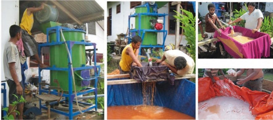
Fig. 17.4 Overall structure of stirrer rotary blade sago starch extraction machine
