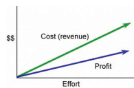
Figure 13.4: In a time-and-materials contract the profit to the contractor increases with increased effort, as does the costs to the client.
