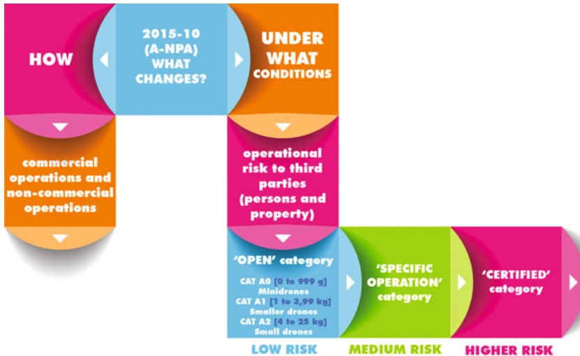
Fig. 2 Changes proposed by the EASA. Source own elaboration adapted from the EASA
