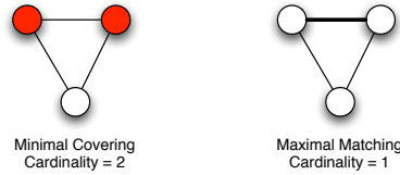
Figure 8.9. In general, the cardinality of a maximal matching is not the same as the cardinality of a minimal vertex covering, though the inequality that the cardinality of the maximal matching is at most the cardinality of the minimal covering does hold.
