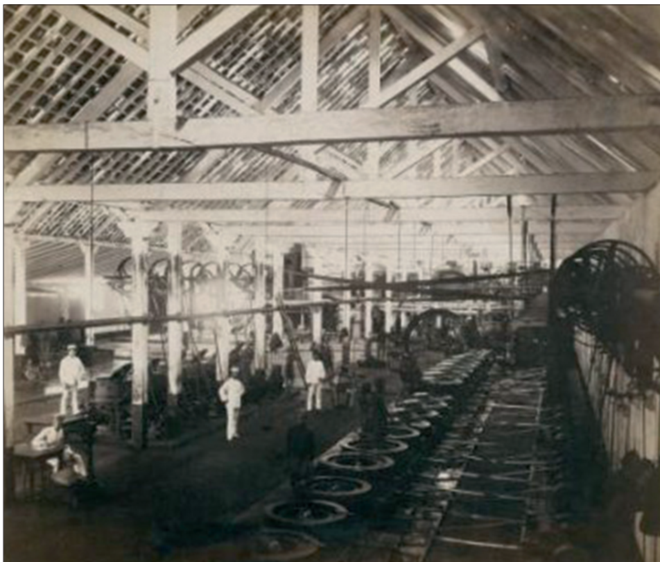
Figure 11: A rare glimpse inside a nineteenth-century Java sugar factory: Pangka, North-Central Java, 1870s. Note the record keeper seated at his table and the (shadowy) presence of Javanese women operating the centrifuges in which half-dry sugar was spun into crystalline form.
