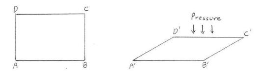
Figure 3. ABCD collapses into A'B'C'D' when pressure is applied.
