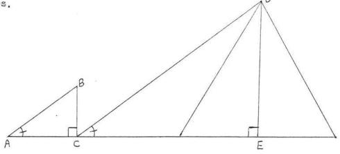
Figure 7. Using similar triangles to measure the height of a pyramid.
