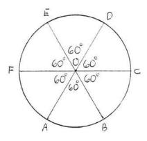
Figure 2. A circle divided into six equal parts.
