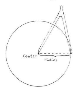
Figure 1. Using a compass to draw a circle.
