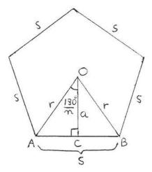
Figure 10. A regular polygon with radius r and side s.
