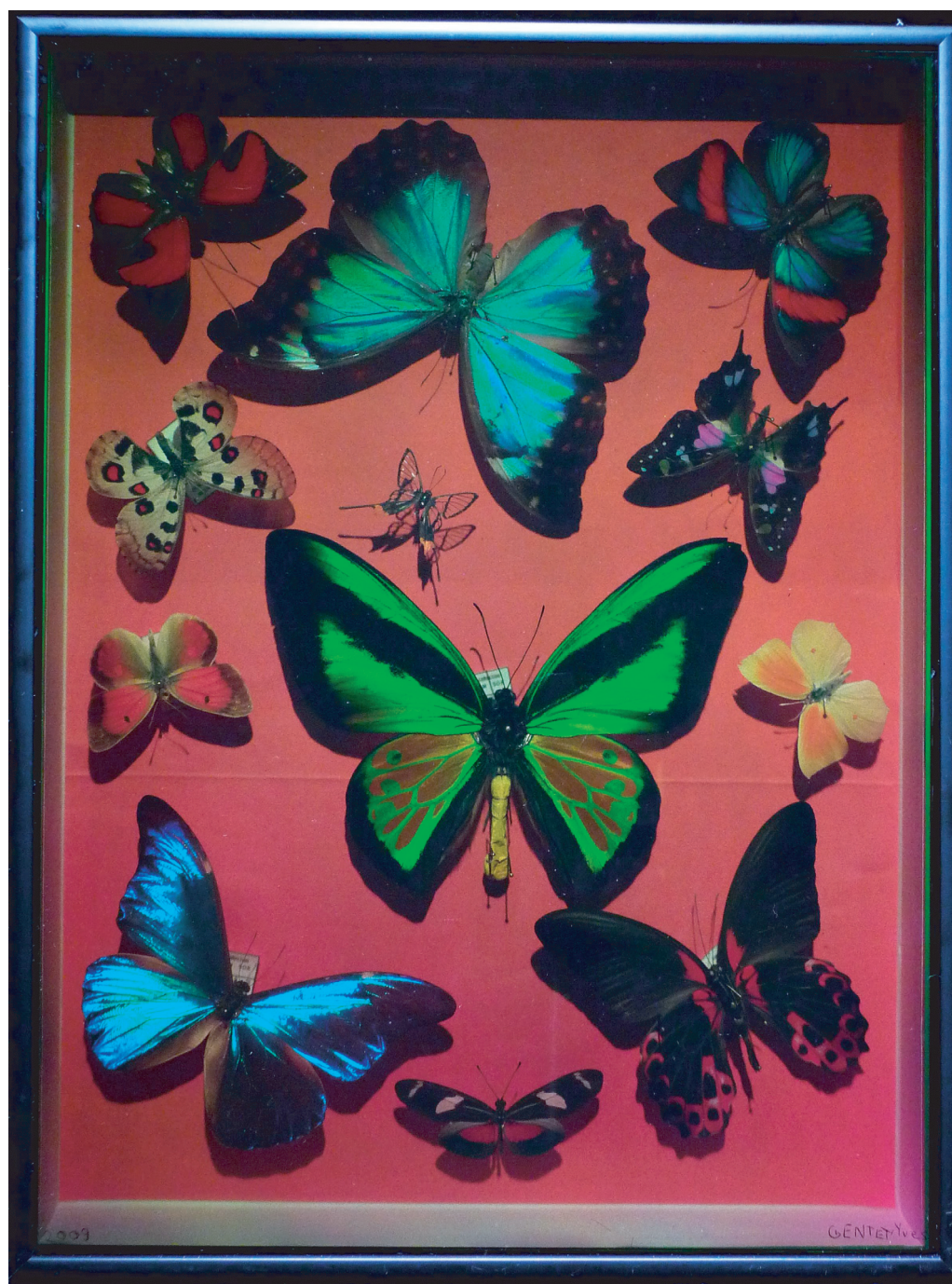
FIGURE 120 The highest-quality holograms available in the world at present are produced by Yves Gentet and can be found on his website www.ultimate-holography.com . They are Denisjuk holograms. The viewer is tricked into thinking that there are real butterflies behind the glass pane. (© Yves Gentet).
