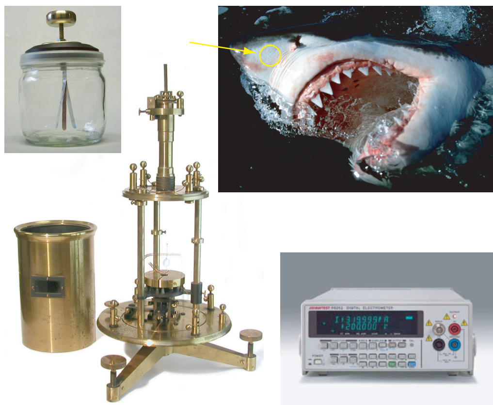
FIGURE 9 Various electrometers: a self-made electrometer based on a jam pot, an ancient (opened) high precision Dolezalek electrometer, the Ampullae of Lorenzini of a shark, and a modern digital electrometer (© Harald Chmela, Klaus Jost at www.jostimages.com , Advantest).
