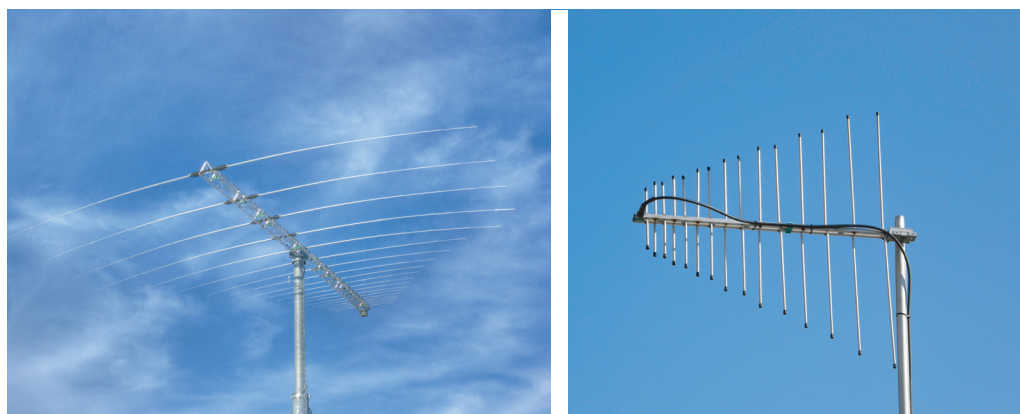
FIGURE 62 Antennas for horizontally and vertically polarized electromagnetic waves (© Martin Abegglen, K. Krallis).
