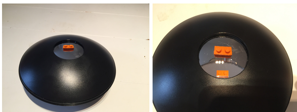
FIGURE 127 A floating Lego brick displayed by two stacked parabolic mirrors, the upper one with a hole. The right picture shows both the brick lying at the bottom and the floating image. (© Christoph Schiller).
