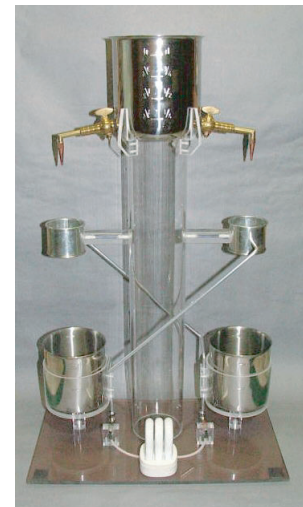
FIGURE 6 A simple Kelvin generator; the one on the right lights a fluorescent light bulb using dripping water (photograph © Harald Chmela).
