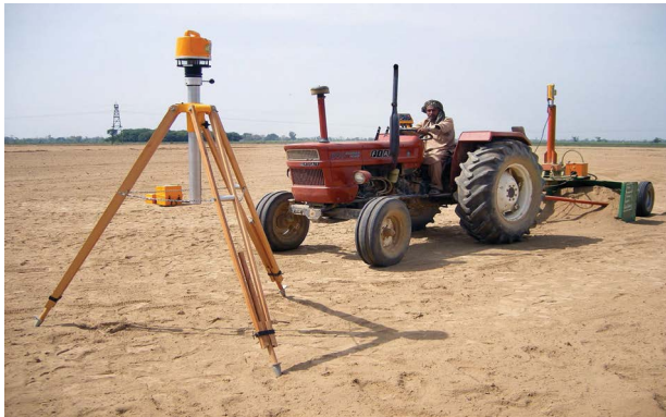
Figure 10: Laser land leveling unit.
