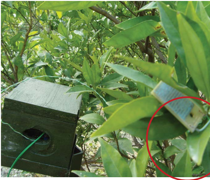
Figure16: Leaf wetness sensor deployment in orange orchard.
