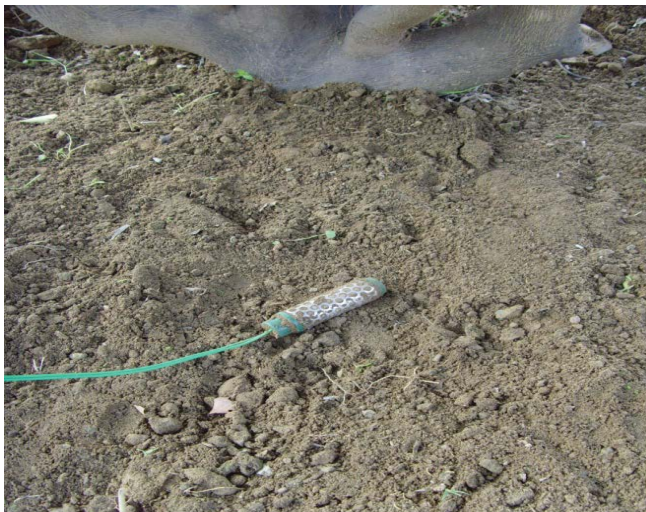
Figure17: Soil moisture sensor deployment near orange plant.
