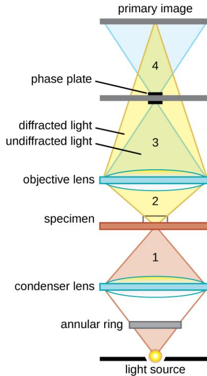
**Figure 1.17** This diagram of a phase-contrast microscope illustrates phase differences between light passing through the object and background. These differences are produced by passing the rays through different parts of a phase plate. The light rays are superimposed in the image plane, producing contrast due to their interference.
