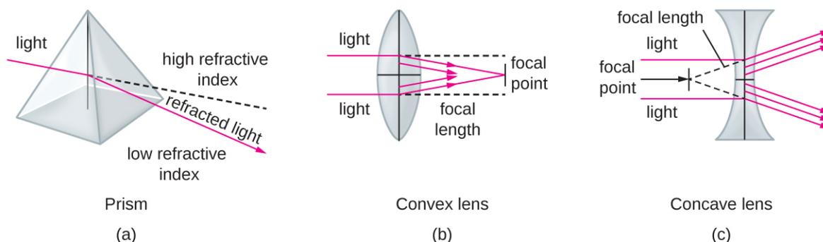
**Figure 1.6** (a) A lens is like a collection of prisms, such as the one shown here. (b) When light passes through a convex lens, it is refracted toward a focal point on the other side of the lens. The focal length is the distance to the focal point. (c) Light passing through a concave lens is refracted away from a focal point in front of the lens.
