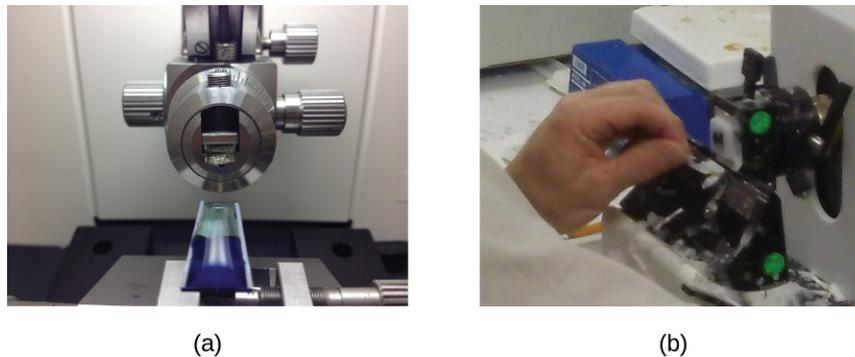
**Figure 1.43** (a) An ultramicrotome used to prepare specimens for a TEM. (b) A technician uses an ultramicrotome to slice a specimen into thin sections. (credit a: modification of work by “Frost Museum”/Flickr; credit b: modification of work by “U.S. Fish and Wildlife Service Northeast Region”/Flickr)
