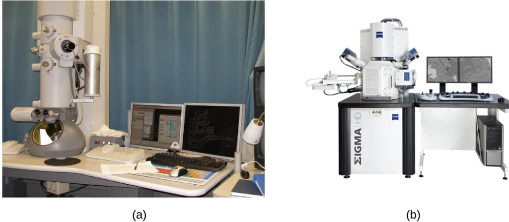
**Figure 1.22** (a) A transmission electron microscope (TEM). (b) A scanning electron microscope (SEM). (credit a: modification of work by “Deshi”/Wikimedia Commons; credit b: modification of work by “ZEISS Microscopy”/Flickr)
