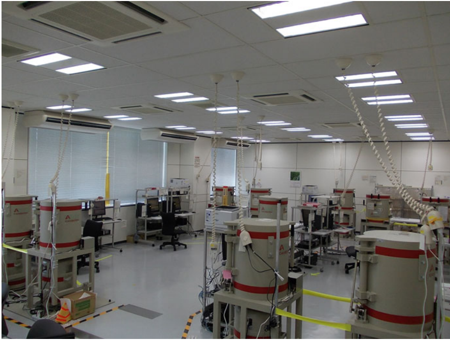
Fig. 8.1 The germanium semiconductor detectors at Fukushima Agricultural Technology Centre
