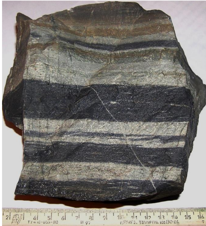
Figure 7.13 Hornfels from the Novosibirsk region of Russia. The dark and light bands are bedding. The rock has been recrystallized during contact metamorphism and does not display foliation. (scale in cm) [ http://en.wikipedia.org/wiki/Hornfels#mediaviewer/File:Hornfels.jpg ]
