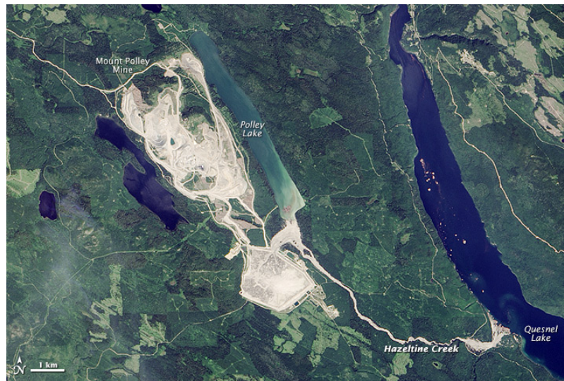
Figure 20.14b The Mt. Polley Mine area after the tailings dam breach of August 2014. The water and tailings released flowed into Hazelton Creek, and Polley and Quesnel Lakes. [ https://en.wikipedia.org/wiki/Mount_Polley_mine_disaster ]
