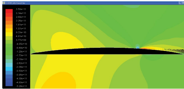
Figure 124: Low pressure is spotted at the upper surface of the Propeller Blade section.
