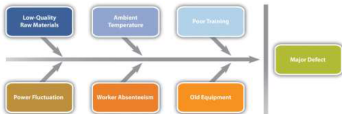
Fig. 10.9: Cause and Effect Diagram Each branch of the diagram can be expanded to break down a category into more specific items.
