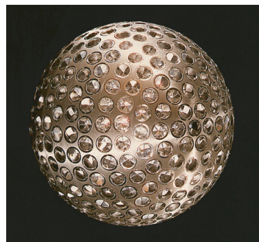
FIGURE 74 The LAGEOS satellites: metal spheres with a diameter of 60 cm, a mass of 407 kg, and covered with 426 retroreflectors (courtesy NASA).
