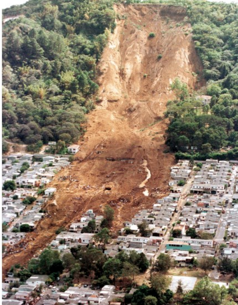
This 2001 landslide in El Salvador (Central America) was started by an earthquake. Soil and rocks flowed down a hillside and swallowed up houses in the city below.
