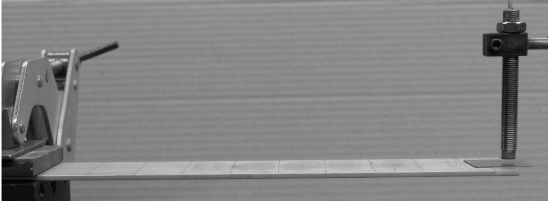
Figure 7-6 Clamped uniform aluminum beam with nominal cross section 2 inch \times 1/8 inch. Test configuration: beam clamped at left between thick steel plates, leaving 10.0 inches of overhang; non-contacting proximity (displacement) sensor over right tip; bonded onto the beam's right tip is a small, thin, steel plate, the "target" in which the proximity sensor induces eddy currents.
