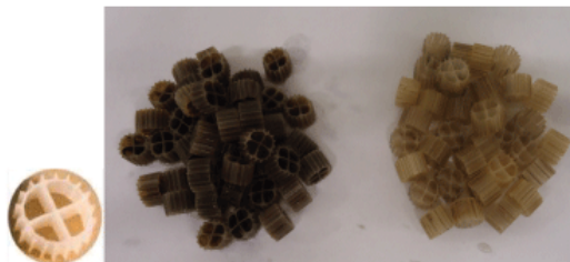
Figure 9: The small and clean biomidia applied for the biofilm improvement and the dirty used biomidias (Anox Kaldnes®), obviously related to the exposure of the biomidia to the effluent, during the treatment proposed studied.
