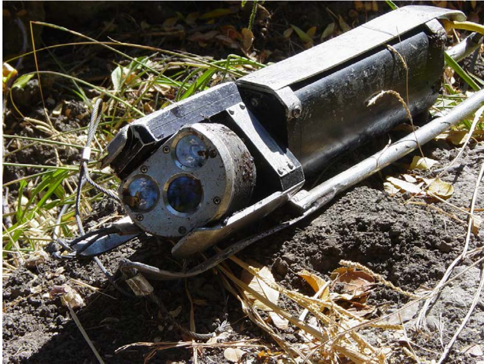
Figure 3.4 - A Video 'Pig' for Pipe Inspection
