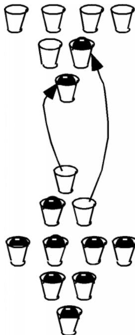
Figure 1.10: Thermal excitation of electrons across the band gap
