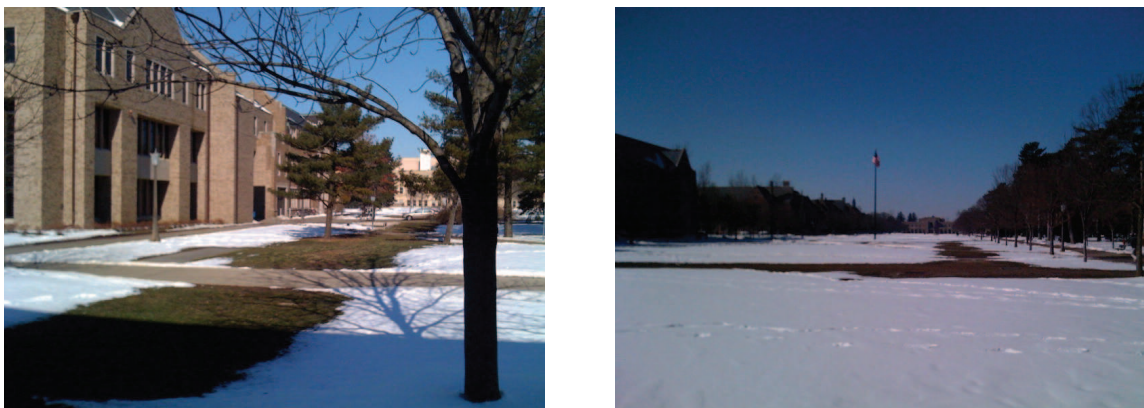
Figure 6.22: Zones of melted snow in regions near underground steam lines on the University of Notre Dame campus, 14 February 2010.
